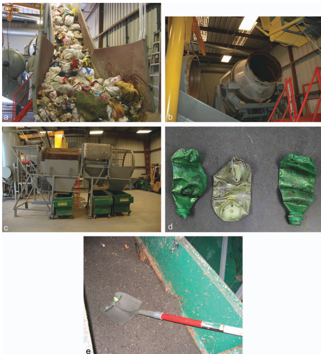
Figure 1 Photographs of PET bottles reclaimed from MSW by vacuum-assisted steam autoclaving. [Color figure can be viewed in the online issue, which is available at wileyonlinelibrary.com .]
